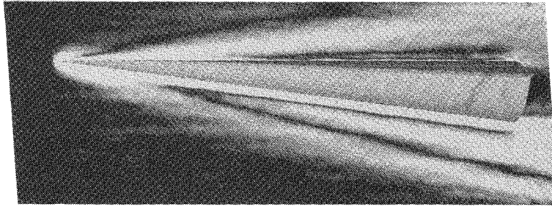
Fig. 11a Density gradient magnitude in the plane of symmetry of waverider at 97 km altitude and 0-deg incidence.
